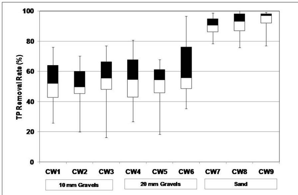
Figure 4. Box plot graphs showing average removal rate of total Phosphorus from dairy wastewater
