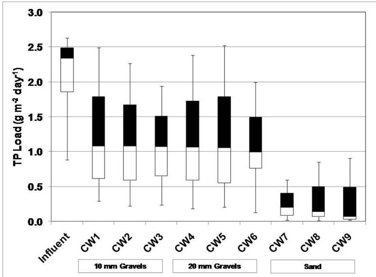
Figure 5. Box plot graphs showing average total Phosphorus load in dairy wastewater
