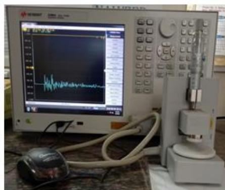
**Figure 3. E4900A Impedance analyser for dielectric analysis**
