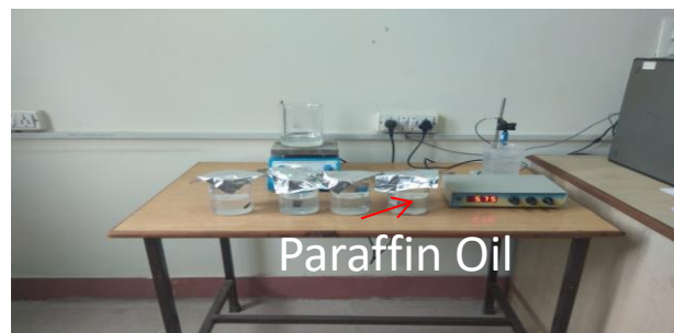
Figure 1. Long term immersion corrosion test representation in sulphide solutions
