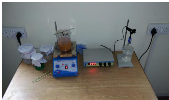
Figure 1. Deposition of CNF nano-particles introduced into EL Ni-P matrix
