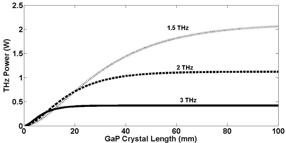
Figure 5. THz power as a function of the crystal length
