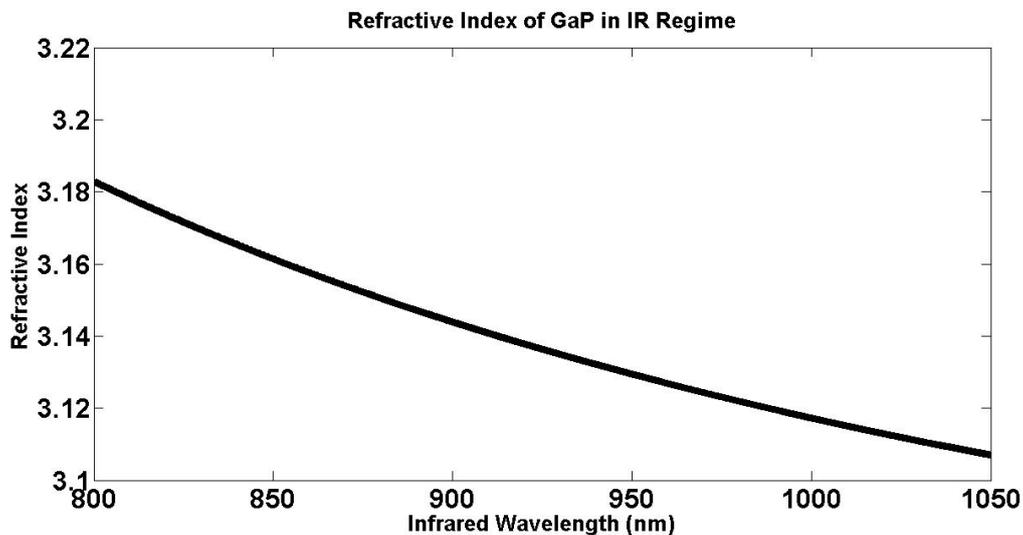
Figure 1. Refractive index of Gallium Phosphide in IR region
