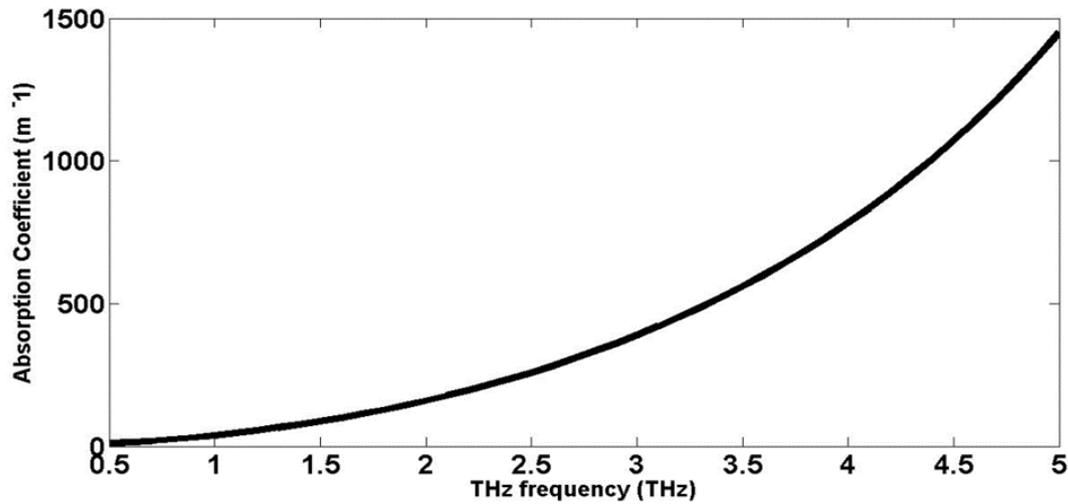
Figure 3. Absorption of Gallium Phosphide in THz region
