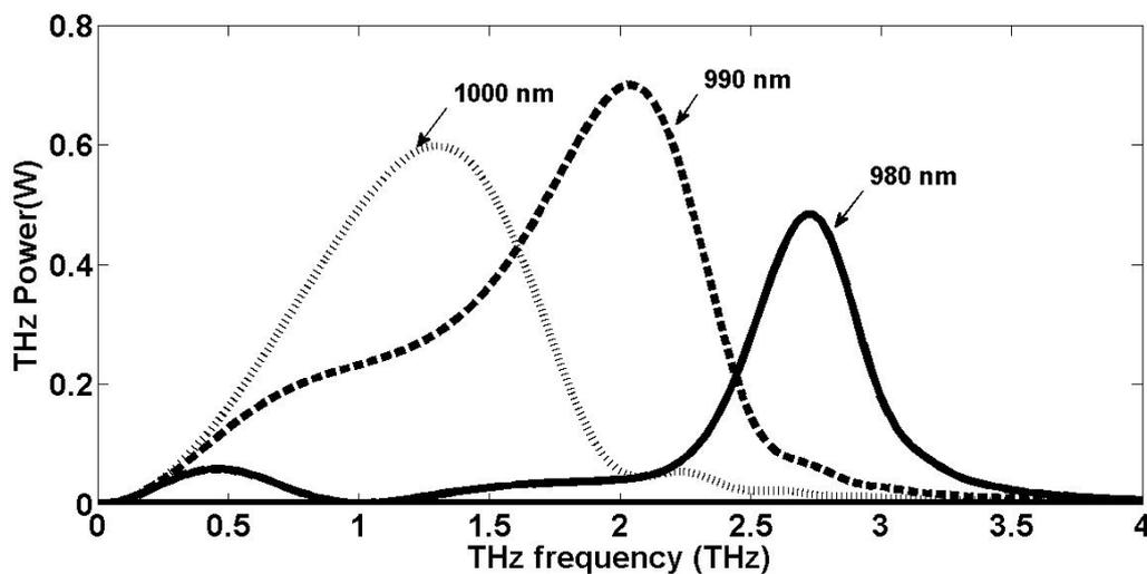
Figure 7. Wider tunability of THz frequency along with the higher output power
