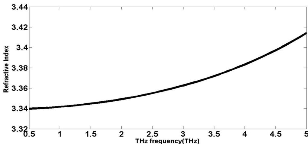
Figure 2. Refractive index of Gallium Phosphide in THz region
